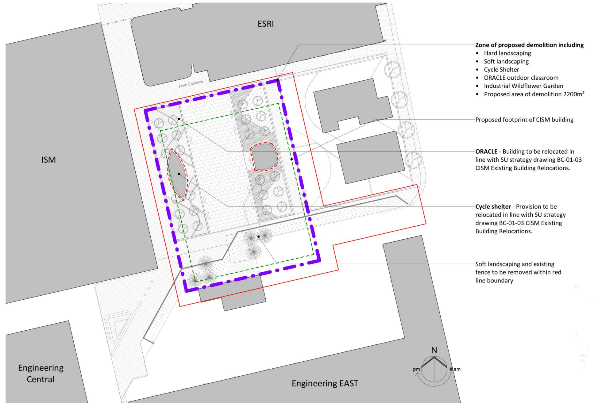
Site Plan. Existing and demolition 1 : 500
